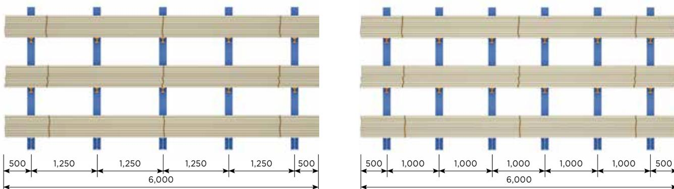
The optimal number of columns to guarantee the resistance and stability of the storage system can vary based on the weight and rigidity of the goods, although their length may be the same.
