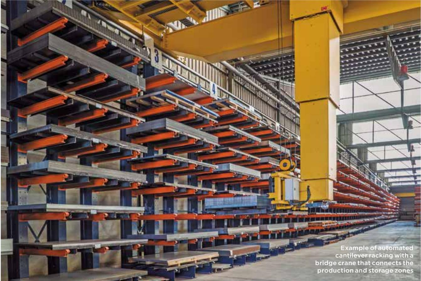
Example of automated cantilever racking with a bridge crane that connects the production and storage zones
