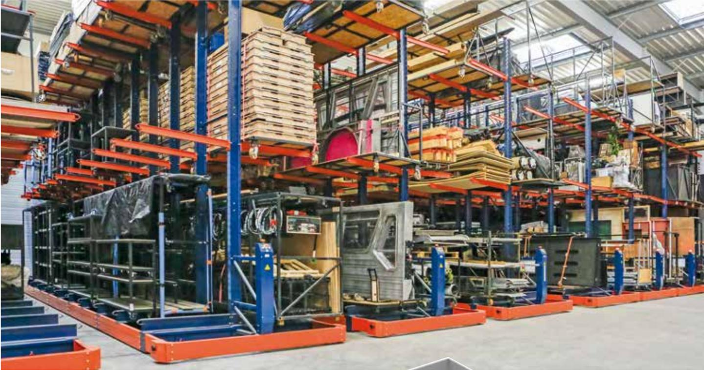
**Cantilever racking on mobile bases**
