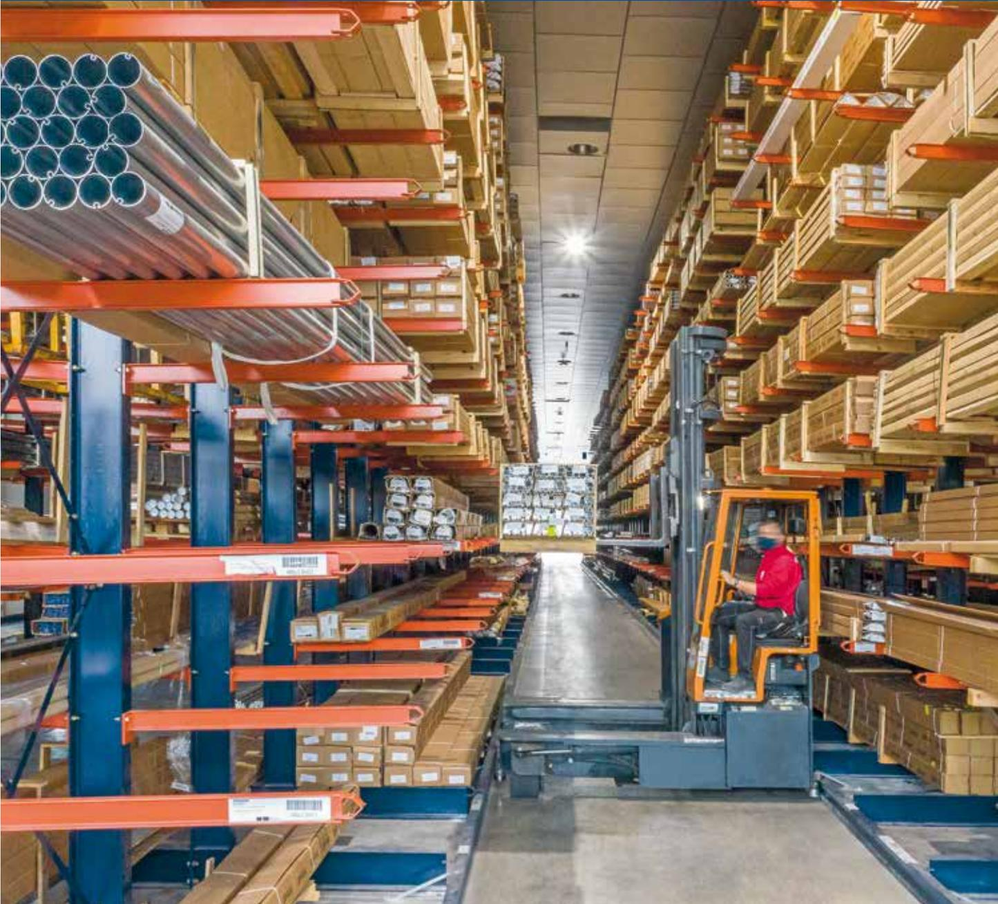
The cantilever racking system consists of different hot-rolled metal profiles developed by Mecalux, with thicknesses and sizes that encompass all market requirements. In order to choose the most suitable system, it is necessary to consider the load weight in addition to the size
