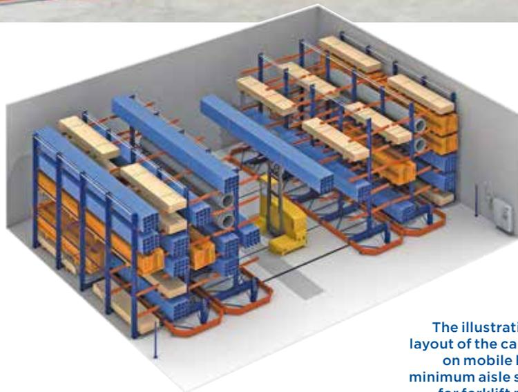
The illustrations show the layout of the cantilever racks on mobile bases and the minimum aisle space needed for forklift manoeuvring.
