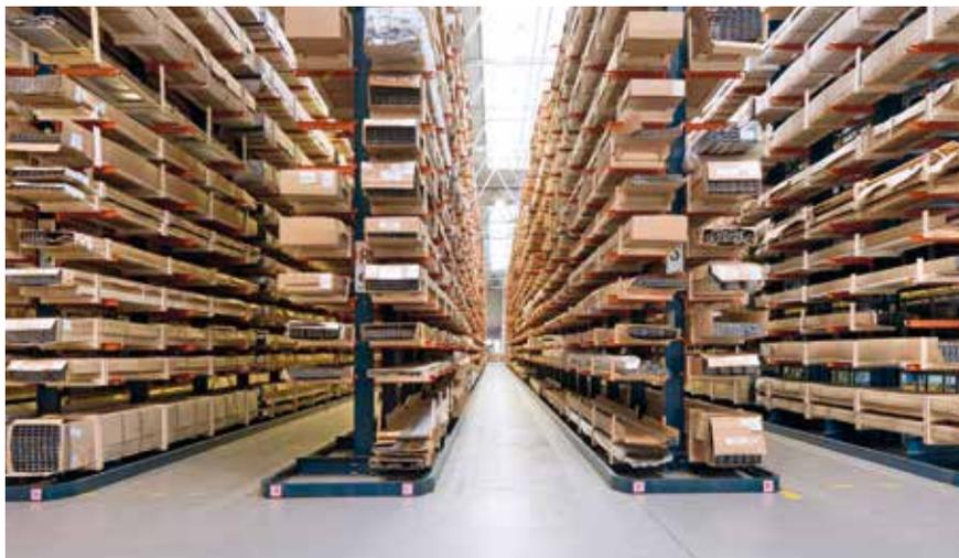
The system comprises vertical profiles (columns) and horizontal profiles strategically positioned to ensure stability. Additionally, overhanging arms are incorporated to support and hold the placed load.
