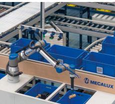
FLEXIBLE SYSTEM CAPABLE OF HANDLING A WIDE RANGE OF ITEMS OF DIFFERENT DIMENSIONS, MATERIALS AND SHAPES.
