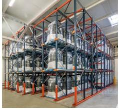
CAN BE USED WITH EITHER LIFO (LAST IN, FIRST OUT) OR FIFO (FIRST IN, FIRST OUT) WITH BATCHES WHEN THERE ARE MORE THAN THREE LANES PER SKU.
