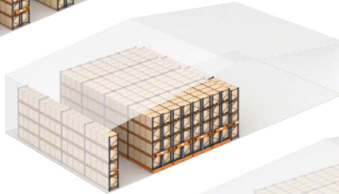
Warehouse using mobile bases. The same capacity with a single aisle occupies less space.
